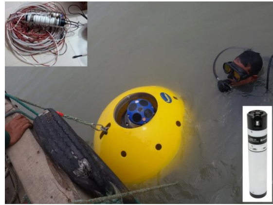
Deployment of the ADCP (inset Turbidity sensor)
